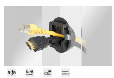
For round metric cut-outs M32/M50 icotek offers the split cable gland with brush strips KEL-BES-S round. It can be either directly snapped into the cut-out or screwed with a locknut, which is included in the shipment.
